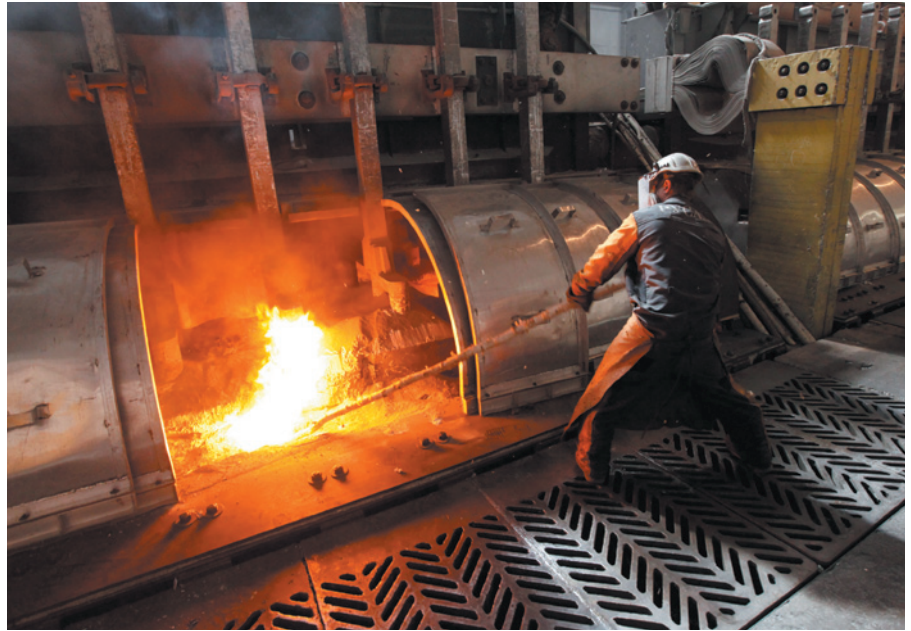
A worker using an electrolysis furnace to produce aluminium in Krasnoyarsk, Russia.
